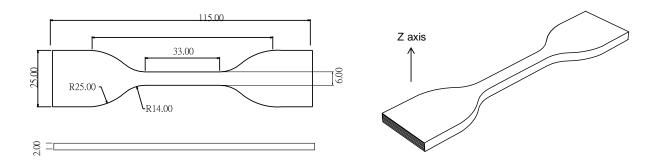
Tensile testing specimen; ISO 37
