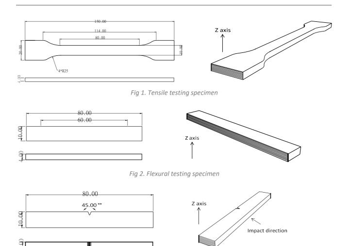
Fig 3. Impact testing specimen
